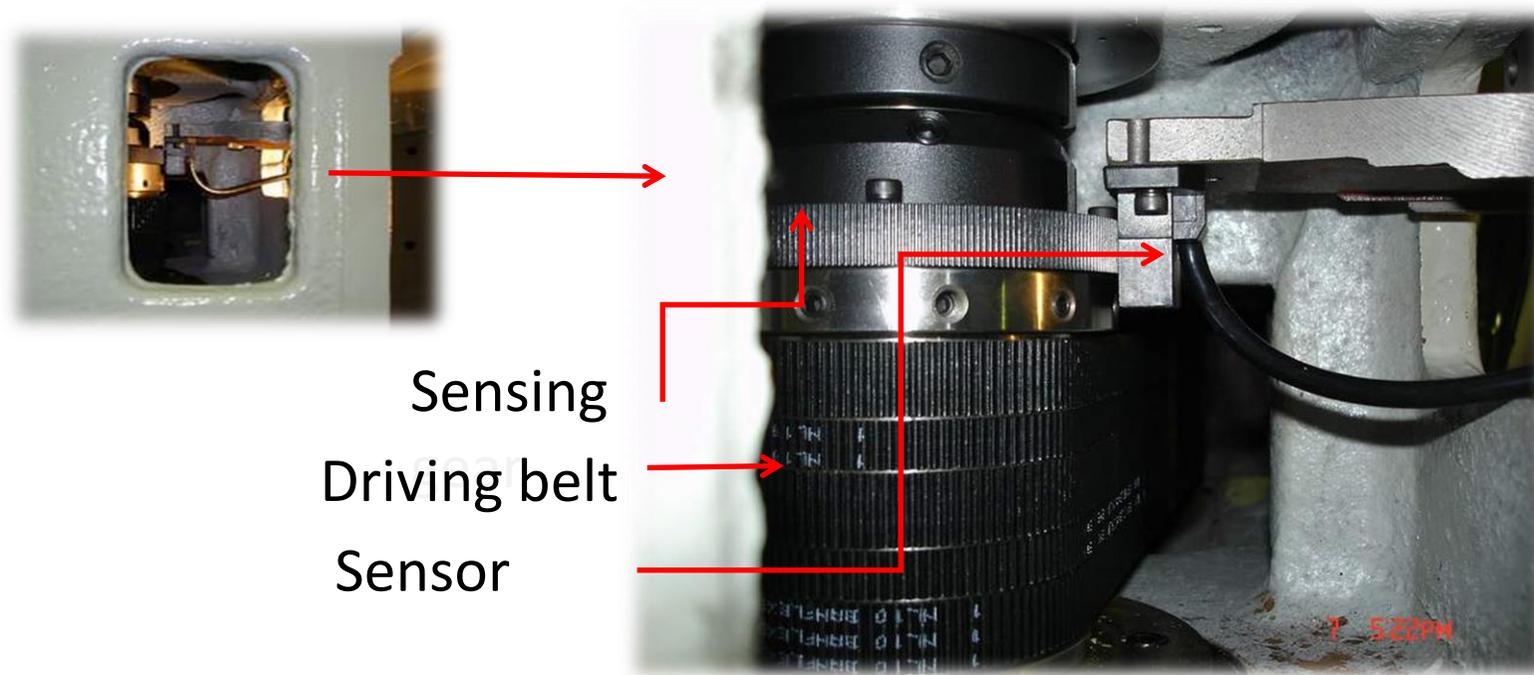
For a Belt-driven VMC. Direct reading spindle position and speed.
