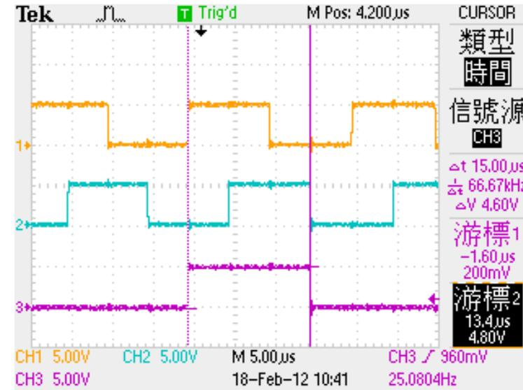
This combination is for a scanning head with a 0.4 mm module and TTL output with 4 fold interpolation with the 0.4 mm module 256 teeth gear wheel. With this selection we can get 1024 output TTL signal
