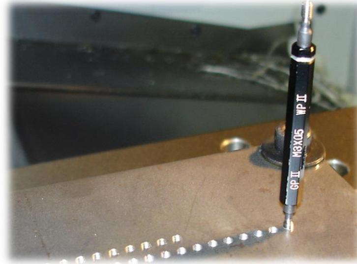
Rigid Tapping in a Vertical Machining Center. When the spindle position is detected directly by a sensor, the belt gear ratio or backlash between motor and spindle will not affect feedback resolution or accuracy ensuring an accurate and repeatable 1.5 ~ 3 mm Rigid Tapping function.
