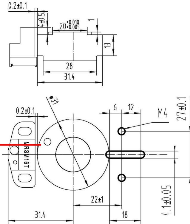
The reference mark label on magnetic ring face up same as Scanning head.
