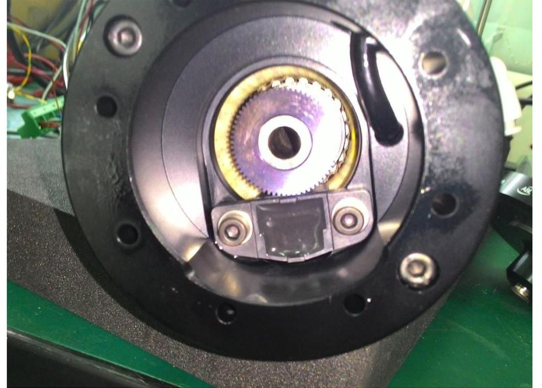
MIS04T04 + 64T gear = TTL 256 ppr = 341.3 KHz
