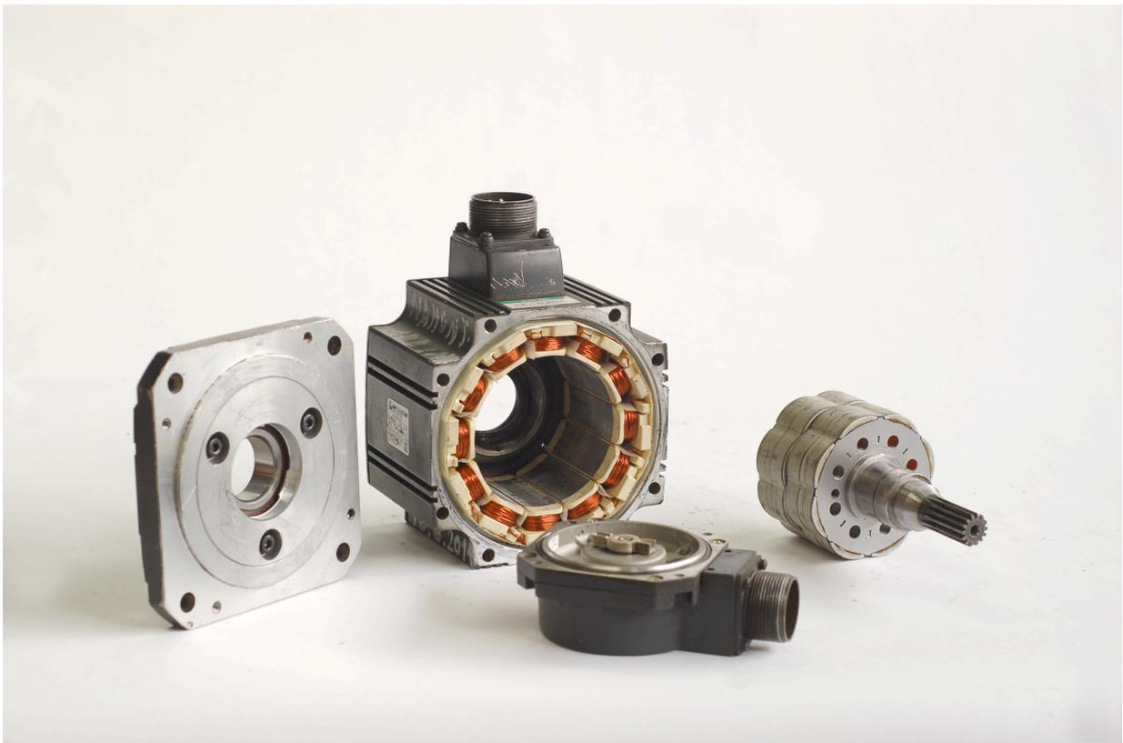
Another feature is that at low speed, maintaining a high torque (N / m) so that it can be defined as a DC motor without brushes.
